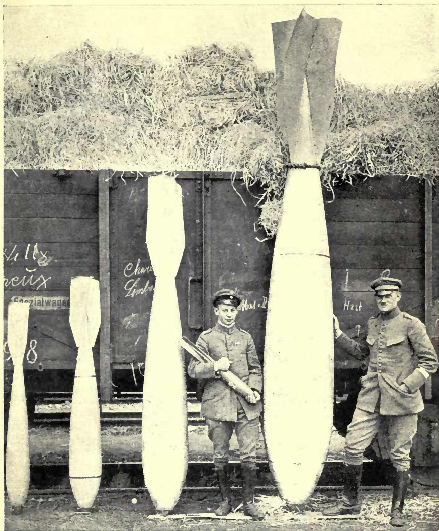
Types of German bombs. From left to right they weigh respectively 110 lb., 220 lb., 660 lb., 27½ lb., and just under a ton. The latter was the heaviest actually used in the war.
