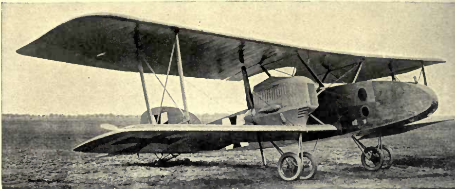
Albatross G 3. Twin engine bombing machine. Crew consisted of rear gunner, pilot, and observer; pilot's seat in centre.
